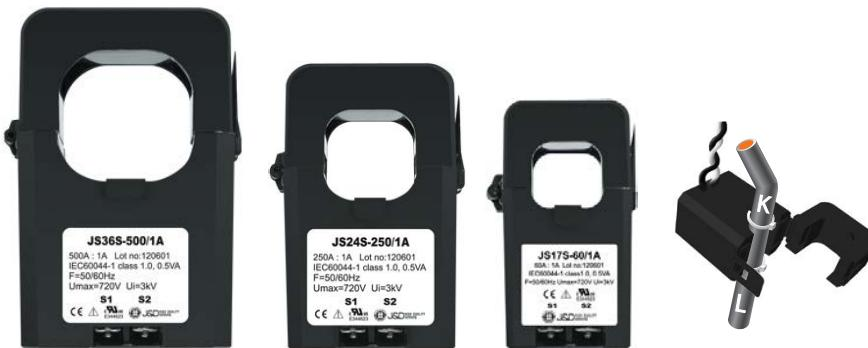
This split-core AC current transformers deliver an output current of 1A from the sensed rated input currents. They are made for watt-hour meters and power meters in power distributions, control panels, switch gears and others appliances. Because of their snap-on design they can simply be turned up on any current-carrying conductor without the need of interrupting the current flow. The built-in output over-voltage protection circuitry allows the secure mounting.
