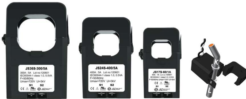
This split-core AC current transformers deliver an output current of 5A from the sensed rated input currents. They are made for watt-hour meters and power meters in power distributions, control panels, switch gears and others appliances. Because of their snap-on design they can simply be turned up on any current-carrying conductor without the need of interrupting the current flow. The built-in output over-voltage protection circuitry allows the secure mounting.
